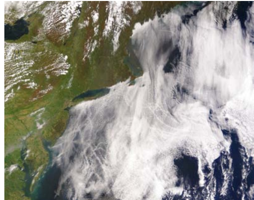
Satellite image of shiptracks (clouds created by the exhaust of ships' smokestacks) over the Atlantic Ocean off the East Coast of the United States. Courtesy of NASA.
